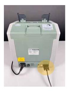
2. The other side of the cable should be connected to the printer.
