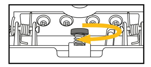
**3(b).** If the unit is experiencing jams or if the bills are getting torn at the input, the feed gap needs to be loosened by turning the knob counterclockwise. Adjust it by a half-turn, then run a test to see if the issue has been resolved. Repeat the adjustment by half-turn increments and testing process as necessary until the unit operates smoothly
