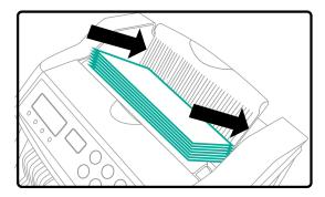
2. Flip the bill stack towards the rear of the machine so the stack is now leaning against the bill guide plate.
