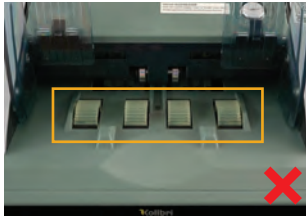
Incorrect roller position.
