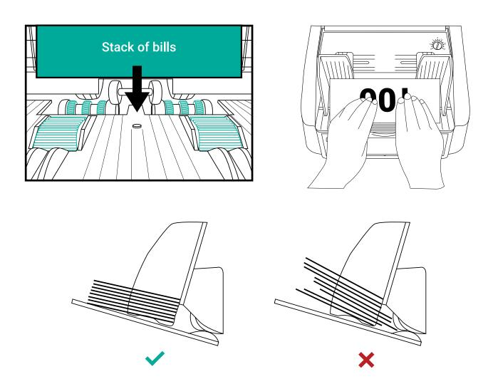
Avoid counting bills that are wet, excessively dirty, soiled, folded, curled or with foreign material like clips, bands, etc. Bills such as these can cause the machine to malfunction.
