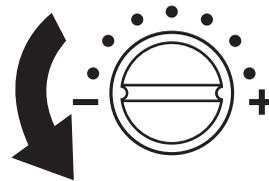
If you are experiencing a high amount of DB, DD errors or multiple bills jammed inside the machine, turn the adjustment screw counterclockwise 2 dots at a time, then retest.
